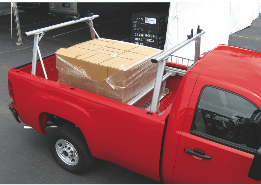
Optional aluminum hardware in this bed includes a load divider, which the 1,300-pound pallet snugs against, and available tool boxes. HD pickups come with 8- or 6.5-foot beds.
