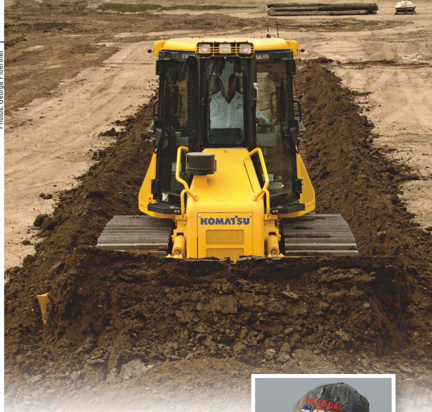
In the slot-dozing exercise, Schultheis was impressed with the D51’s ability to keep a large load rolling.
