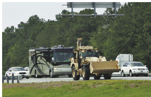
The JCB HMEE, equipped with four-wheel anti-lock air brakes, is capable of towing up to 10,000 pounds.
