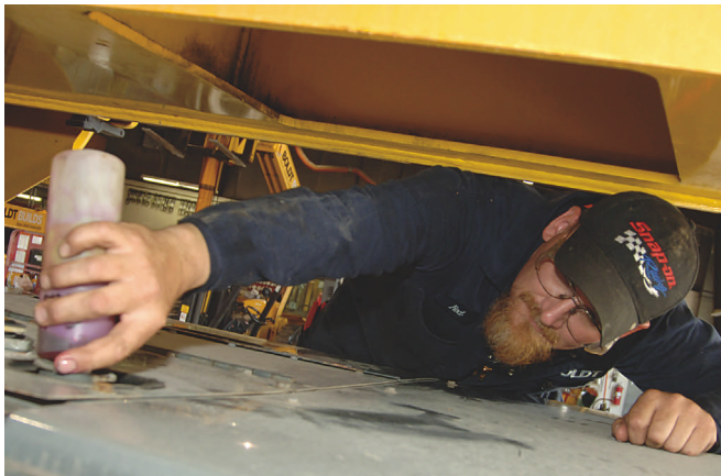
For The Boldt Co., the move to increasingly place equipment decisions where the actual work is located is a major adjustment for a company with a long history. Here, Rod Kent, Local 139 operating engineer and mechanical technician, fills and checks fluids on a Grove rough-terrain crane.
